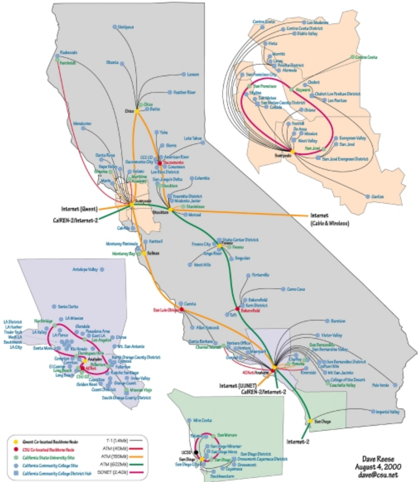
Figure 4. 4CNet Network Topology
